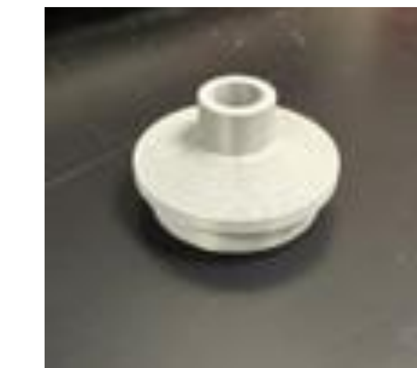
Figure 8. FlexiValve Inhaler Cap (3D-Printed)
