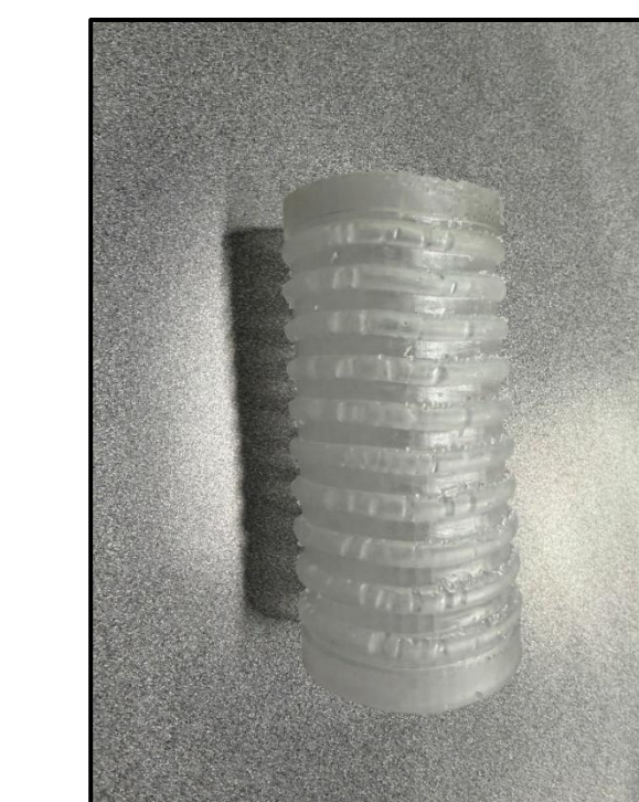
Figure 9. FlexiValve Chamber Body (3D-Printed)
