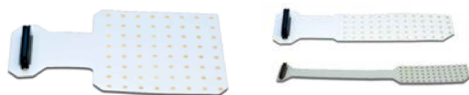
Figure 2: The 8x8 electrode array (2 were needed) and the 2 different sizes of the 5x13 electrode arrays
