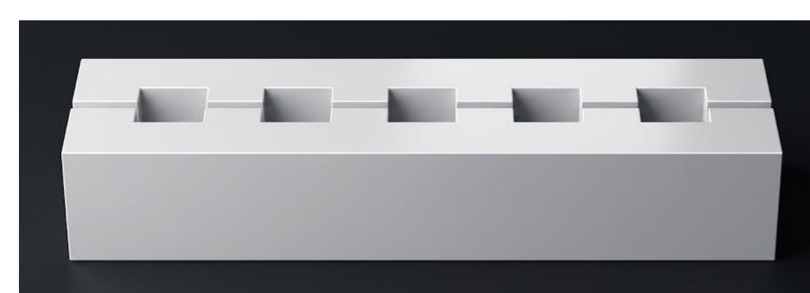
Figure 2: Custom 3D-printed V2 casting molds (125 \mu L cavity) featuring a central trench to accommodate the surgical thread backbone.
