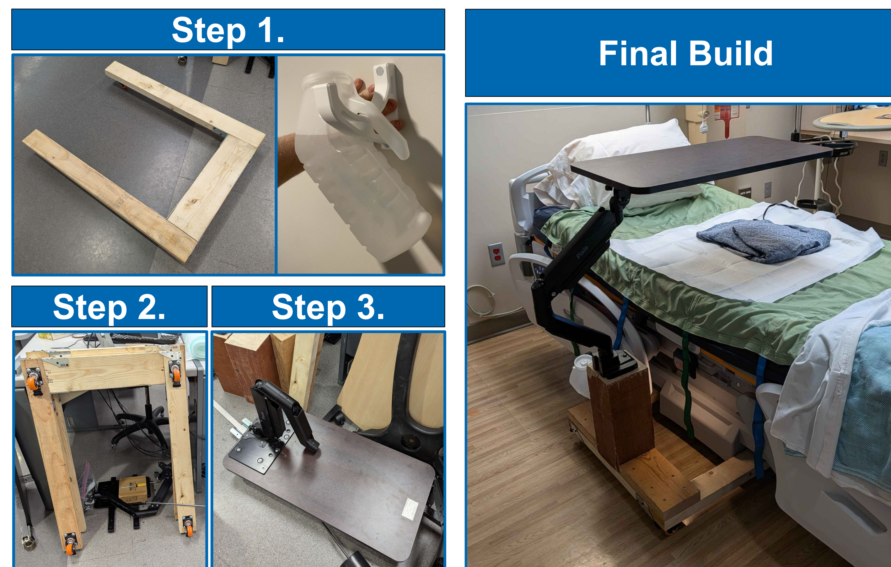
Figure 3. Alpha prototype constructed out of a wooden base and adapting articulating monitor arm. Key innovations are a new set of casters, a beam-mounted urinal bottle hook, and additional rotational degree of freedom for improved handling. Future iterations will add a storage compartment, a cupholder, and a lip to prevent spill overflow.
