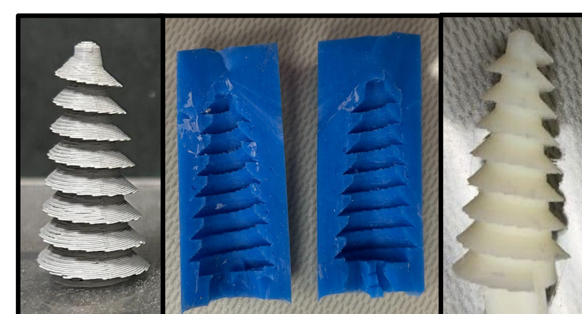
Figure 7: 3D print, silicone mold of print, polyurethane prototype.
