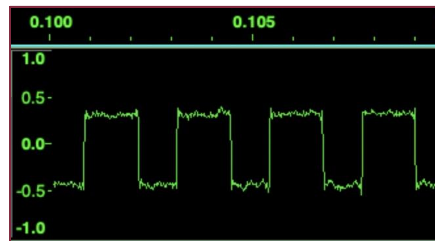
Fig. 3: PWM Switching Waveform from Oscilloscope Image Credit: Trumpetep, Wikimedia
