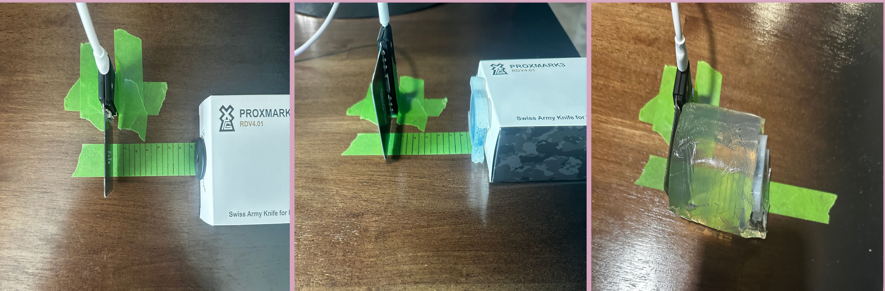
Figure 5. Read Distance Testing in Air and in Ultrasound Phantom.
