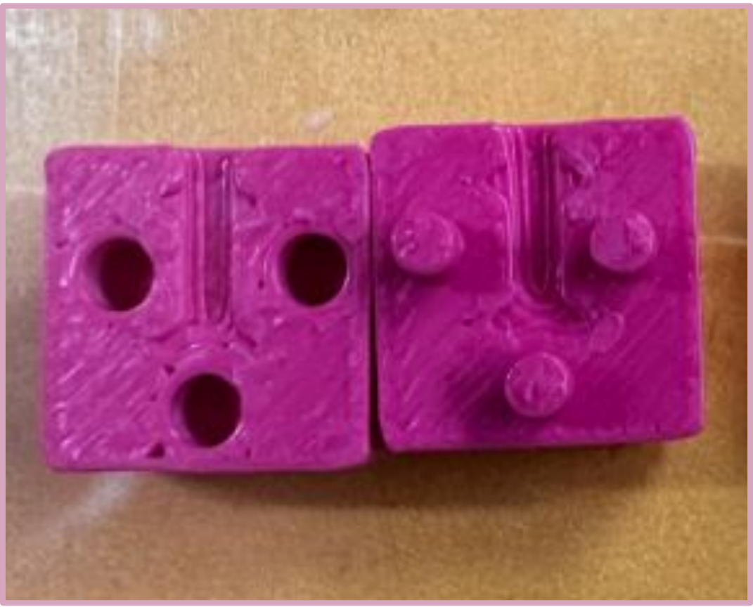
Figure 1. Final Design of Mold for Silicone Blank.
