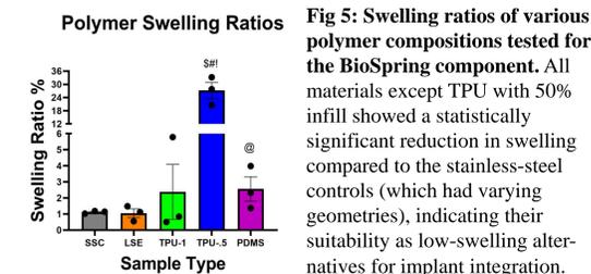
**Fig 5:** Swelling ratios of various polymer compositions tested for the BioSpring component. All materials except TPU with 50% infill showed a statistically significant reduction in swelling compared to the stainless-steel controls (which had varying geometries), indicating their suitability as low-swelling alternatives for implant integration.
