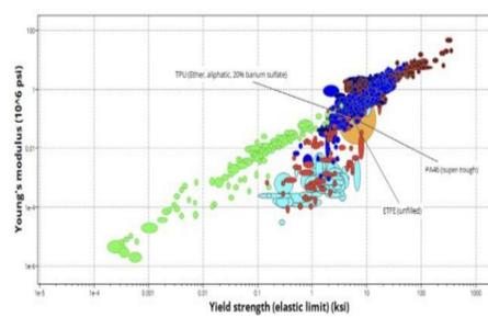
**Fig 3.** Material Selection Process via Ansys Granta EduPack. TPU 20% Barium Sulfate hit the desired yield strength metrics with 98% similarity. Soft polymers were selected due to similar mechanical properties with a larger range of compressibility.
