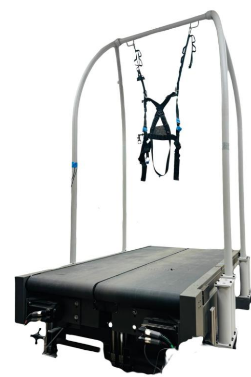
Figure 1. . Experiment layout of treadmill for reactive balance experimentation
