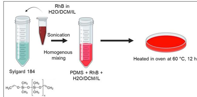
PDMS films were prepared by mixing Sylgard 184 base with curing agent at a 10:1 ratio.
