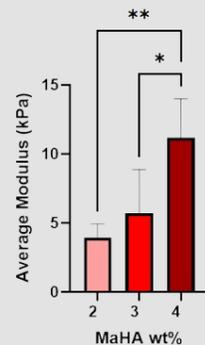
Figure 9: Compression testing data run on MaHA hydrogels are varying weight percentages (2, 3, 4wt%) showing an increase in weight percentage increases the average elastic modulus of the MaHA hydrogel.
