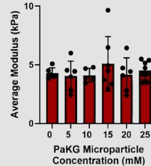
Figure 11: Compression testing data run on 2 wt% MaHA hydrogels with varying amounts of paKG MPs (0, 5, 10, 15, 20, 25mM) showing the addition of paKG does not impact the average elastic modulus of the MaHA hydrogel.
