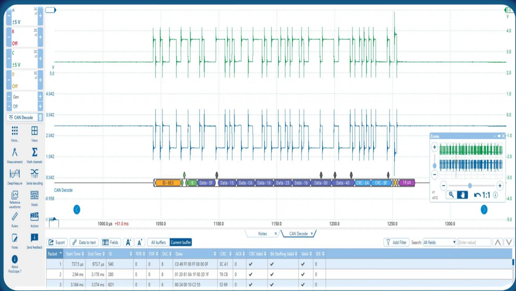
FIGURE 1: DECODING DIFFERENTIAL CAN FRAMES
