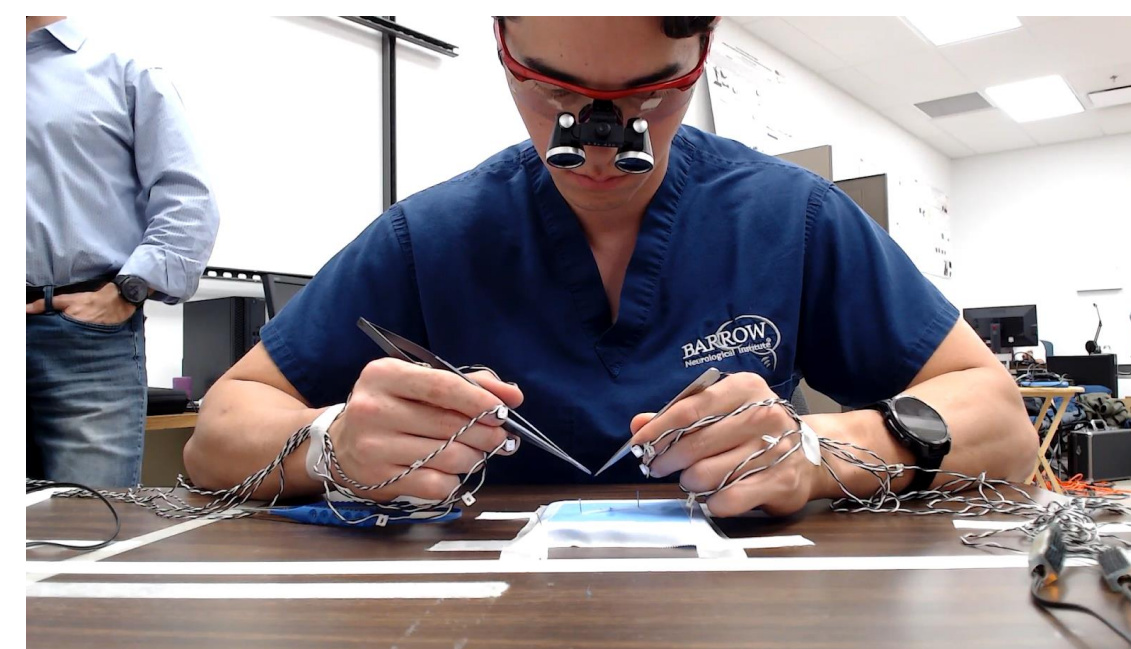
Figure 2: Thomas, a medical student is performing neurosurgical suturing with 1 marker on each finger (10 markers total), tracked by 10 PhaseSpace IR cameras for movement analysis.
