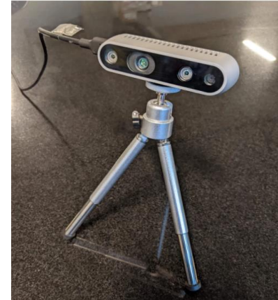
Figure 2: The Intel camera with built-in stereo cameras and IR sensor that will be used to track hand movements for markerless system through Google's MediaPipe.
